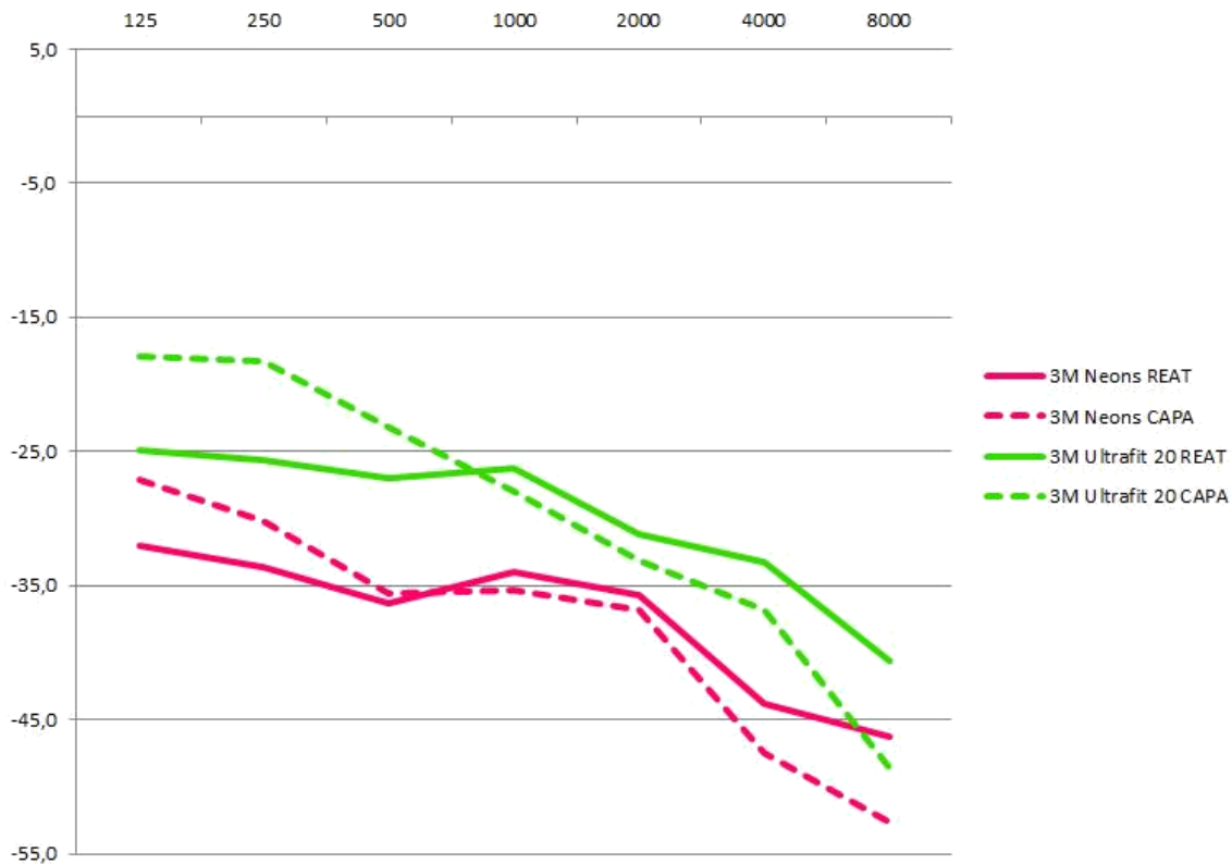
Figure 2: Comparing the measurements of the CAPA system with the reference values of the REAT method for a preformed earplug, Ultrafit by 3M, and an ear cap requiring shaping by Neons by 3M
