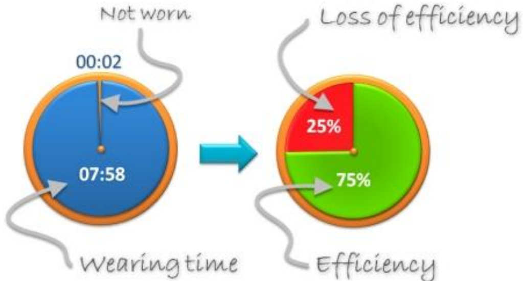
Loss of efficiency of the HPD when it is not worn (Example 2) [4]
