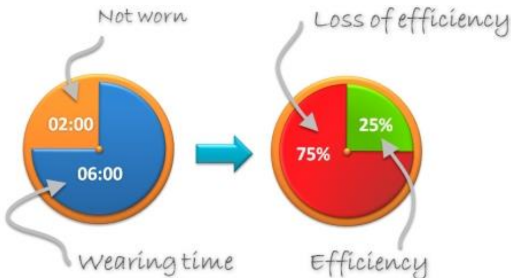
Figure 15: Loss of efficiency of the HPD when it is not worn (Example 2)
