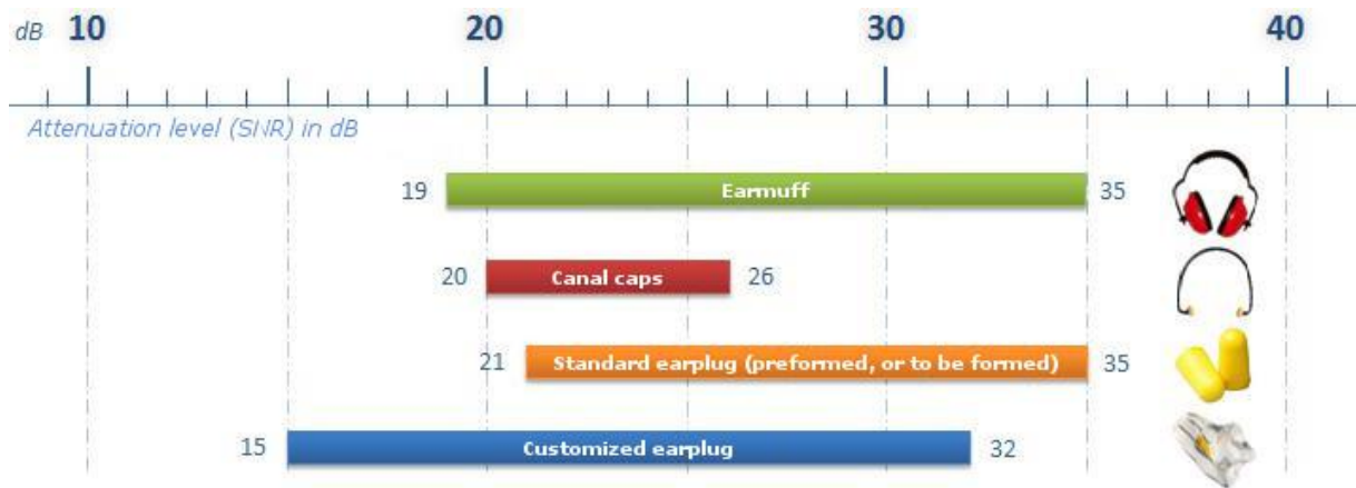
Graph 6: Theoretical attenuation ranges (laboratory measurements) of different HPDs
